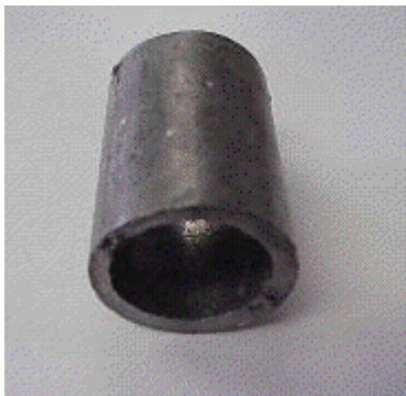
Pipes with lead
