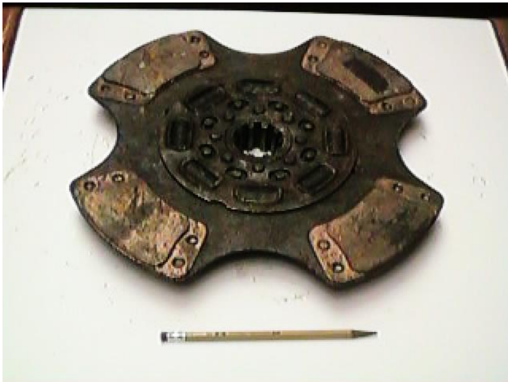
Clutch Plate with Copper Metal Pads
