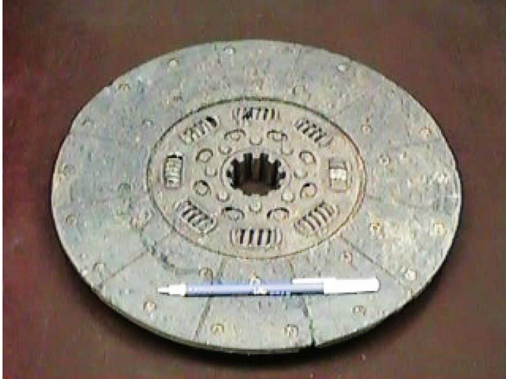
Clutch Plate with Copper- or Brass-Impregnated Non-Metallic Pads
